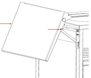
4. To lock the shelf in place, pull the shelf / strut assembly up, and pivot the shelf down and onto the shelf pins. The shelf should sit firmly on the pins, and with the strut fully lowered in the bracket slot.
